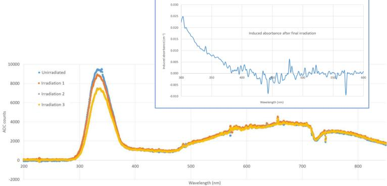
The result of a three-day continuous gamma irradiation, to a total dose of approximately 0.44 kGy, of a 3 mm diameter silica rod. Data are dark count corrected [3]. The transmission dip near 725 nm is due to the 40 m of high-OH silica fibre in the total light path.
