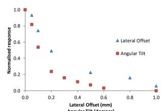
Fibres are illuminated by a combined deuterium and halogen light source focussed onto the end of the fibre with a 0.25 NA radiation-tolerant quartz lens. Light transmitted by the fibre is collected by an identical lens and measured as a function of wavelength with a linear CCD spectrometer covering a wavelength range of 190 to 850 nm. We simulated the sensitivity to misalignment using ZEMAX [2]
