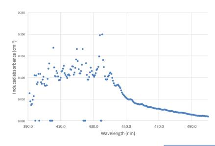
The result of a four-day continuous gamma irradiation, to a total dose of approximately 10 kGy, of a 3 mm diameter commercial polymethyl methacrylate (PMMA) rod that was highly absorbing prior to irradiation at wavelengths shorter than 390 nm due to a UV absorbing additive.
