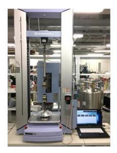
**Figure 4.** Universal mechanical testing machine (AG-X plus, SHIMADZU Co., Ltd., Kyoto, Japan) for conducting tensile tests.
