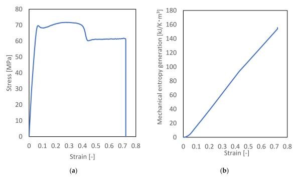
**Figure 5.** (a) Stress–strain diagram of PA6 obtained experimentally from the tensile test and (b) mechanical entropy generation, calculated using experimental data.
