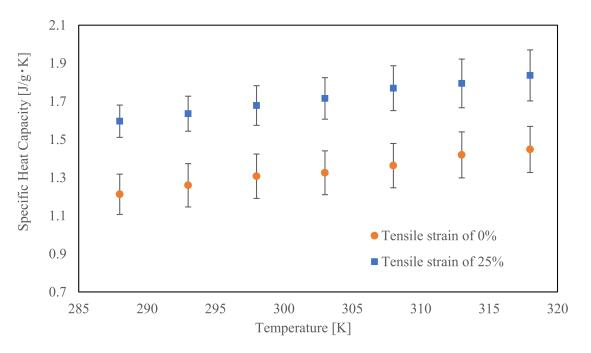
Figure 6. Relationship between the tensile strain and specific heat capacity.
