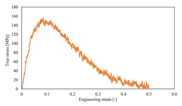
Figure 2. Stress-strain curve of PA6 obtained using MD simulations.
