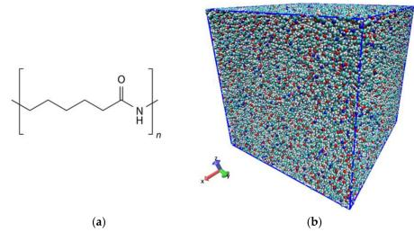
**Figure 1.** Illustration of (**a**) chemical structure of PA6, and (**b**) the initial system of PA6 consisting of 1000 molecules.
