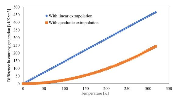
**Figure 8.** Thermalentropy generation before and after tensile deformation with linear and quadratic extrapolation.
