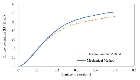
**Figure 3.** Fracture and thermal entropy generation of PA6 during tensile analysis using MD simulations.
