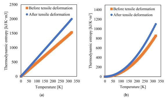
**Figure 7.** Thermalentropy generation before and after deformation, calculated using (**a**) linear and (**b**) quadratic extrapolation of the specific heat capacity.
