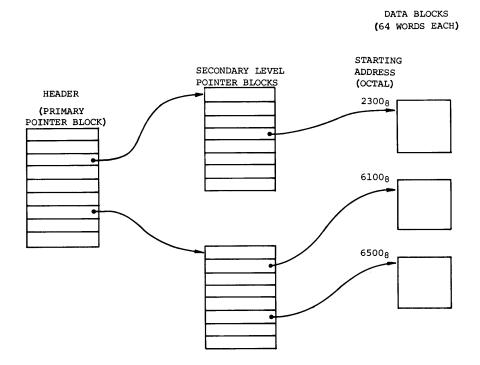
Figure 1: Example of an ECS file, with three existing data blocks and a maximum possible size of 4608 words.
