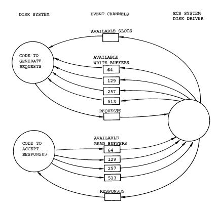
Figure 3: Sketch of event flow between disk system code and ECS system disk driver.
