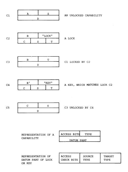
Figure 7: Example of locking and unlocking.
