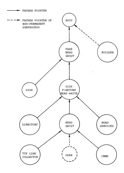
Figure 5: The subprocess tree of a user process.
