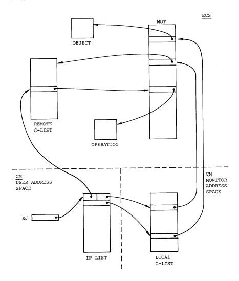
Figure 6: Pointer structure for a typical ECS system call, with an indirect reference to the operation.
