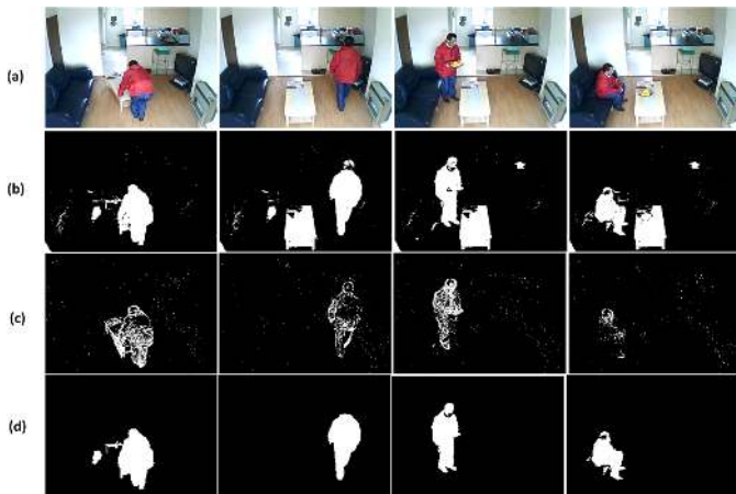
Fig. 11. Background subtraction results for moving furniture. Line (a) shows original frames of a person moving the table and fruit plate. Codebook background subtraction results are shown in line (b). Line (c) shows the frame differencing results which indicate active pixels. From the frame differencing results and blob operations, improved background subtraction results are obtained in line (d).
