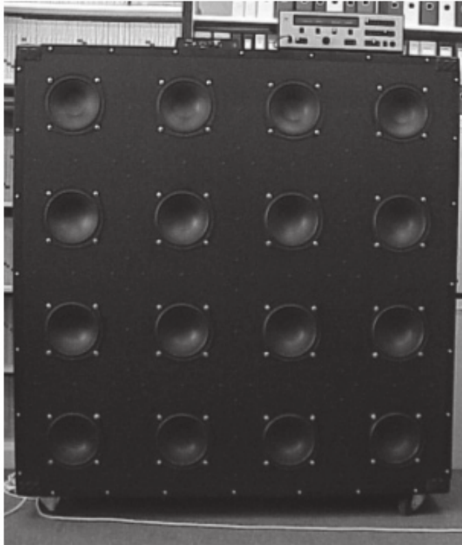
Figure 7. An acoustic model of a power transformer.
