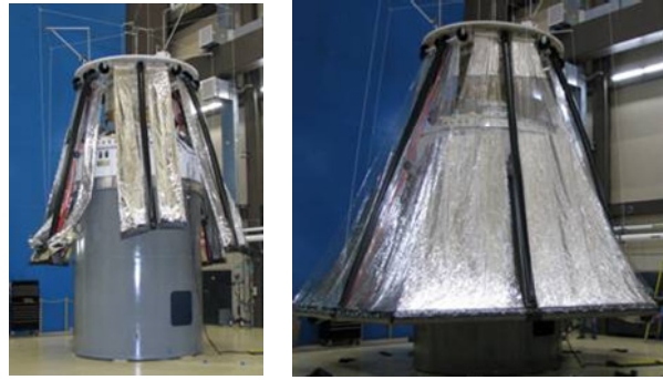
Figure 15. ULA is developing a pneumatically deployed sun shield to support long duration cryo storage.
