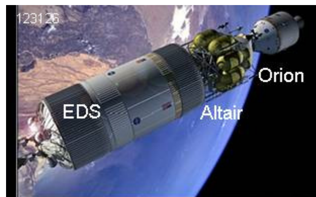
Figure 2. The EDS helps loft Altair to LEO and then accelerates the Orion-Altair combination to Earth escape. Credit: NASA
