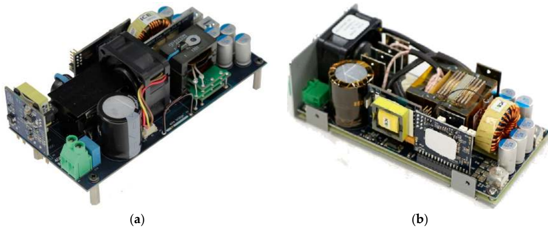
Figure 20. Prototypes of PSFB DC-DC converter for server applications: (a) original reference design; (b) optimized design.
