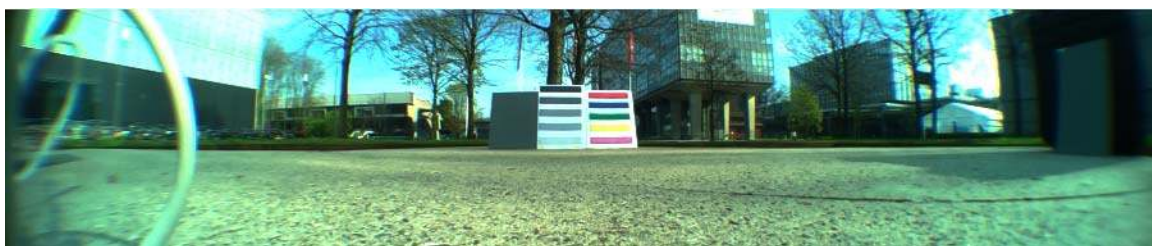
Fig. 9. Setup for the accuracy measurements. Gray and colored targets were placed in the center of the image and one gray target was placed at the border. The accuracy was determined by comparing luminance measurements with the calculated luminance, this was repeated for multiple conditions.
