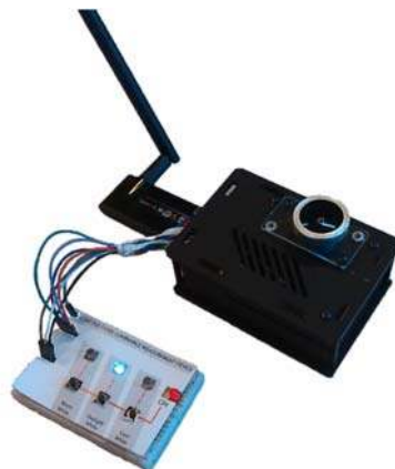
Fig. 1. The measurement device, including a Raspberry Pi 2, Camera Board, fisheye lens, dongle, and control panel (see section 2.4)
