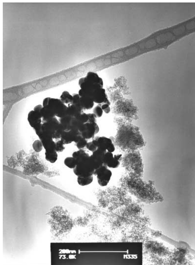
Figure 1. TEM picture of palladium (black circles) deposited on silica from Heck reaction.
