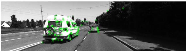
FIGURE 17: ORB-SLAM2 extraction of features from moving vehicles. This causes an altered ego-motion perception which leads to incorrect odometry estimates.
