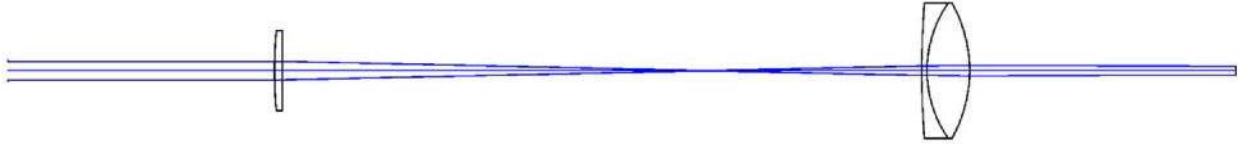
Figure 35. 2D layout of the system. The beam is clearly reduced in size and not perfectly collimated (i.e., weakly focusing).
