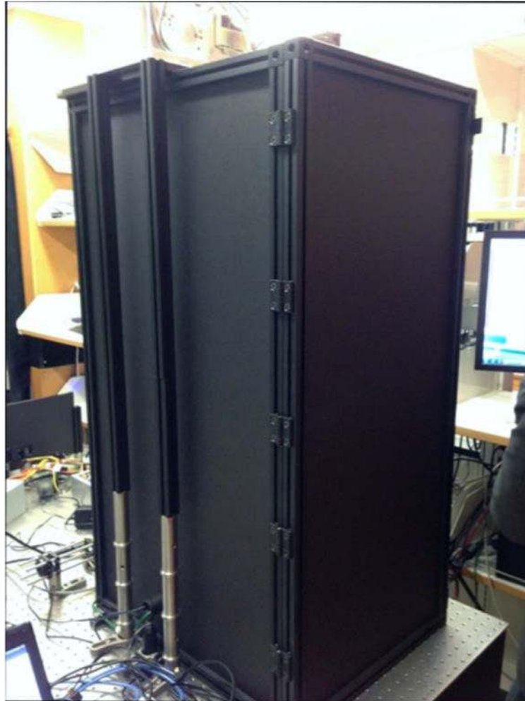
Figure 79. Microscope fully enclosed. The 12" \times 18" breadboard (MB1218) is mounted on top of the enclosure to support the scan mirror electronics. The supports visible on the side have been added to secure this breadboard.
