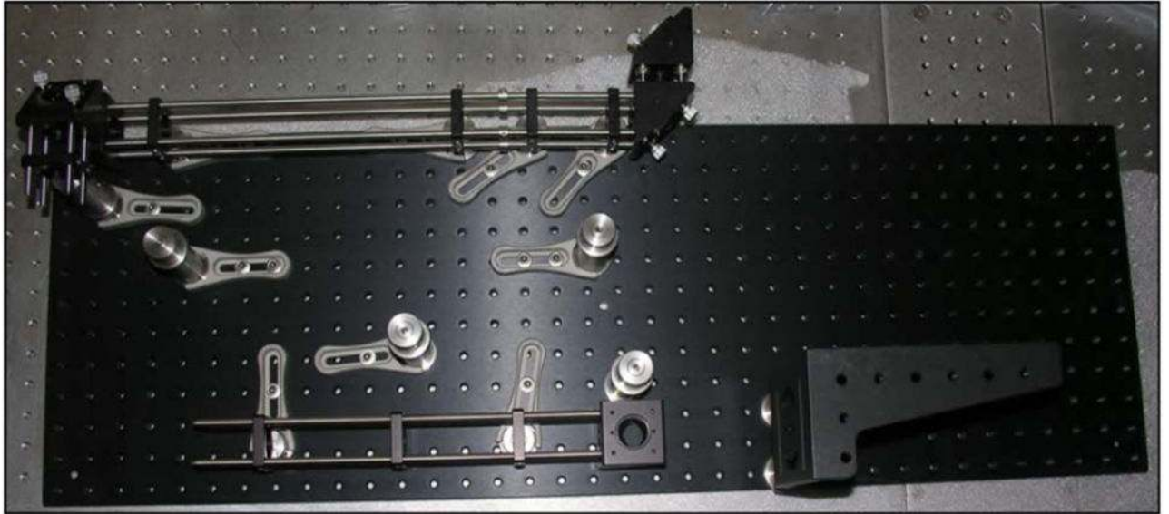
Figure 69. Step 8. Third caged optical system added and secured to pedestal (upper left in image). Caged kinematic mirror mount, four 2" rods, and one 30-mm cage plate (CP08).
