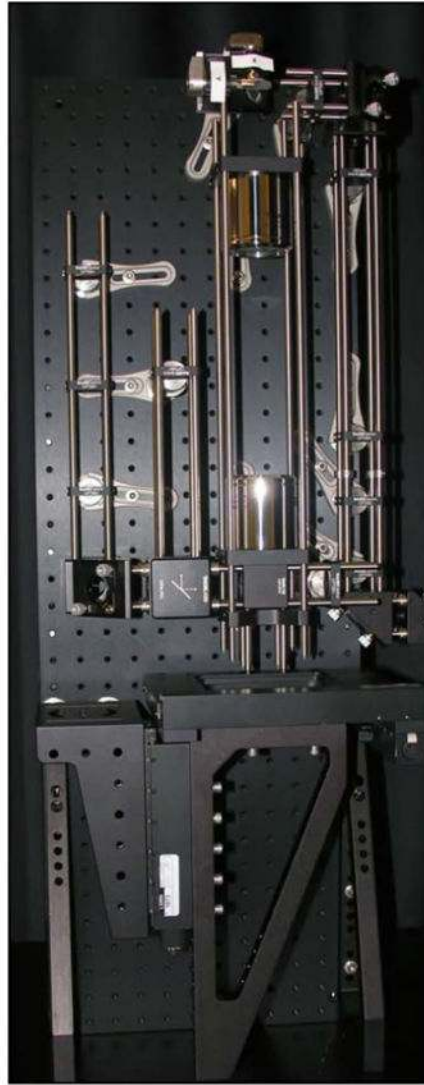
Figure 78. Step 17. Scan optics and scan mirrors added.
