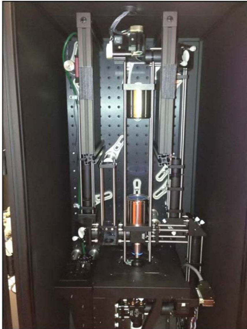
Figure 80. Inside view of the enclosure with a fully functional microscope. PMTs (beneath the stage) and a white-light camera (red module in upper left of image) have been installed. The beam tubes and additional baffles are visible.
