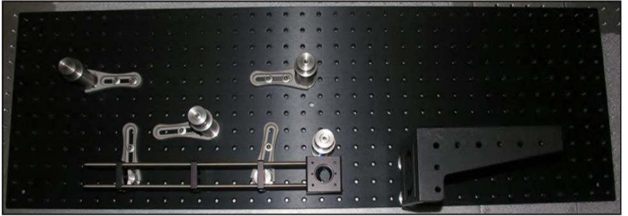
Figure 66. Step 5. Four pedestals with clamps added to host the next level of caged optics.
