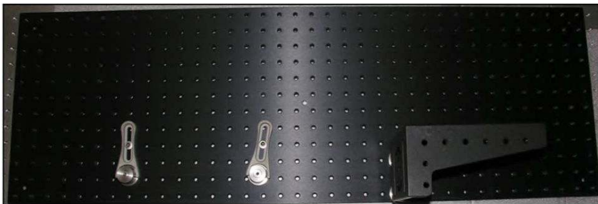
Figure 64. Step 3. 1"-high 8-32 pedestals and clamps are added.
