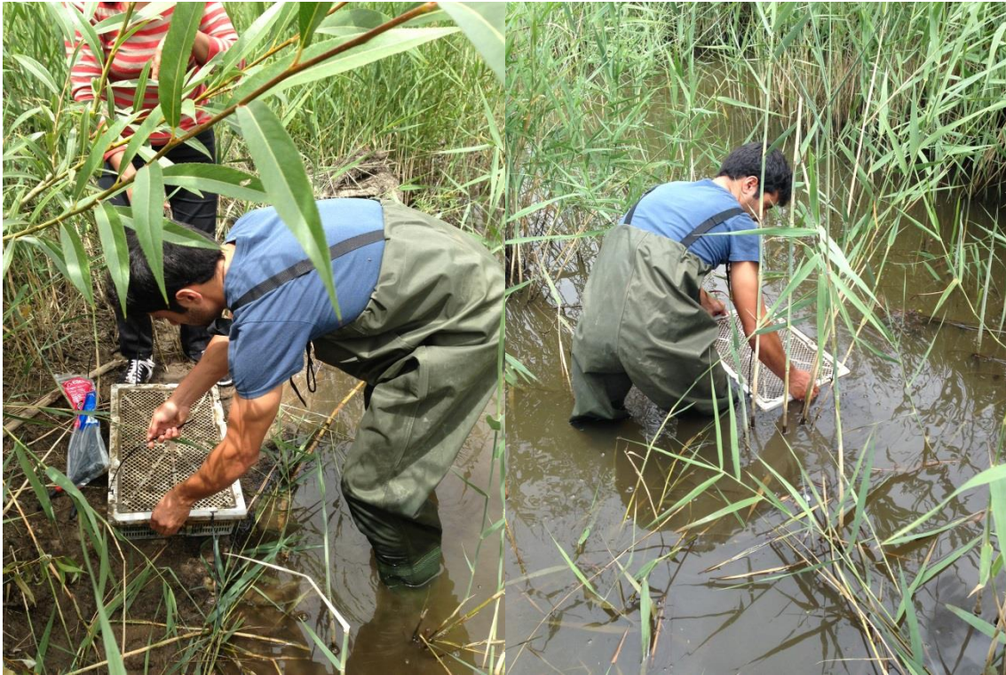
Figure A3.1 Plastic cages (2 cm mesh) used to for the in situ bioassay.
