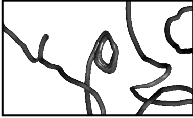
Figure 4. Vortex skeleton at time 194.4 located by the predictor-corrector method. Note the spiral in the center.
