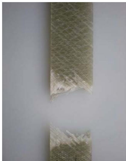
0.81% Initial strain, R = 0.1 # of cycles to failure 52,041 (a)
