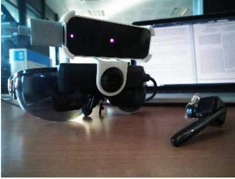
Fig. 2. Leap Motion Controller, Vuzix AR Glasses and Plantronics Headset
