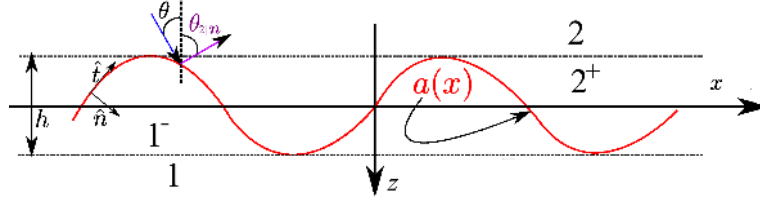
Fig. 31. Grating geometry and different regions referred in the text. Graphene follows the profile a(x) .
