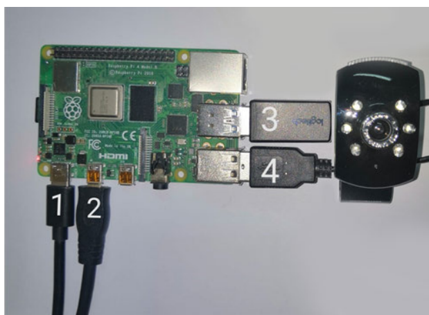
FIGURE 9. The Raspberry Pi 4 with camera attached to the main board.
