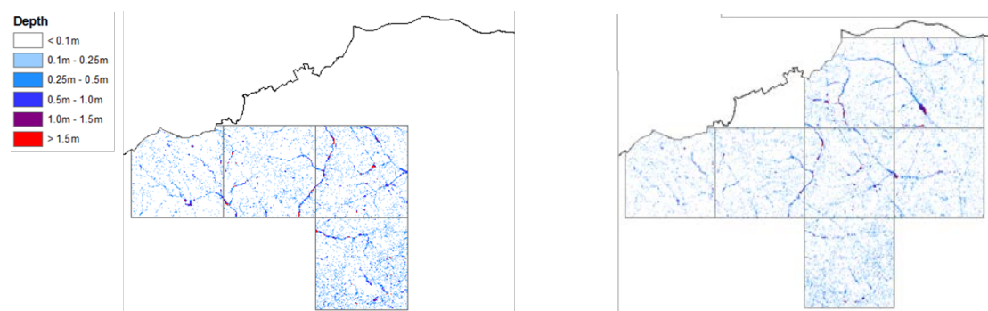
Fig. 6: Synthetic surface water flood outlines corresponding to the events shown in Fig. 4.
