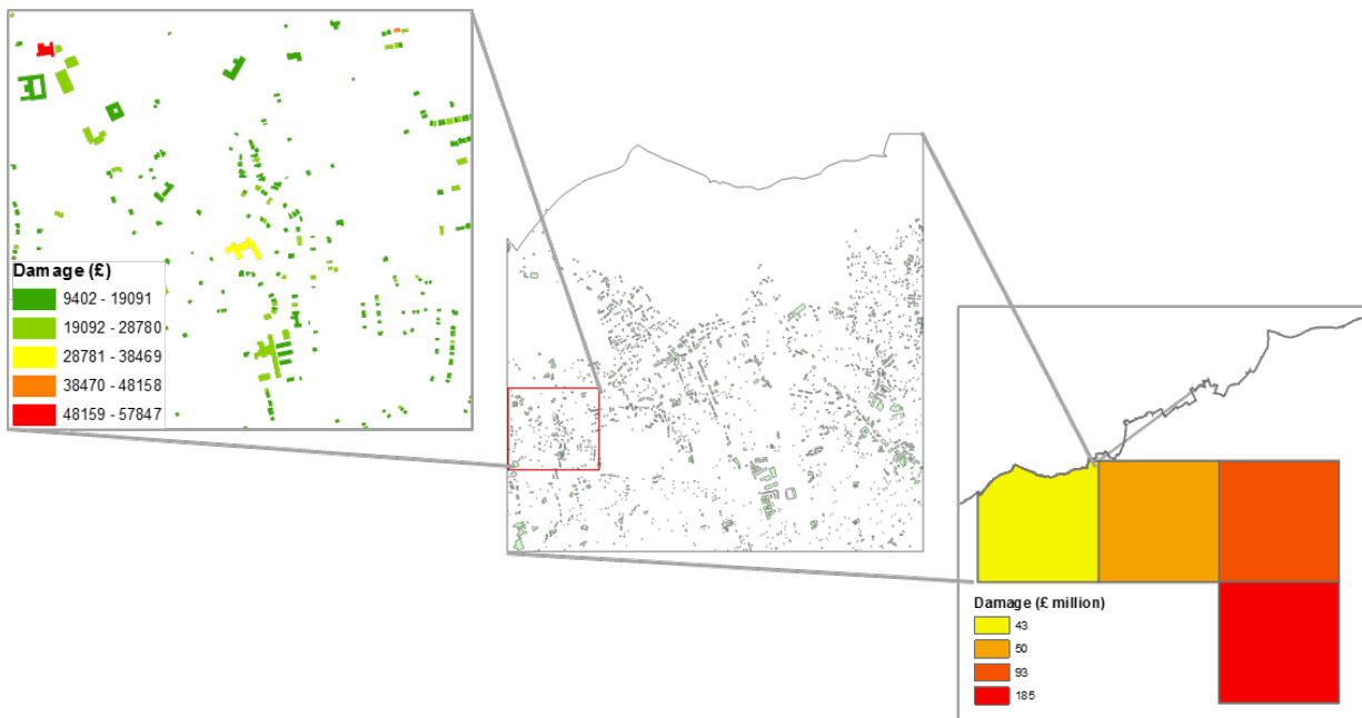
Fig. 9: Left panel: Estimated damage to a sub-set of residential properties at risk of flooding during a 1/100 yr event and the damage per property. Middle panel: Spatial footprint of all properties at risk in one grid cell based on the synthetic flood outline. Right panel: The total damage per grid cell for the event (corresponding to the flood outline shown in Fig.6).
