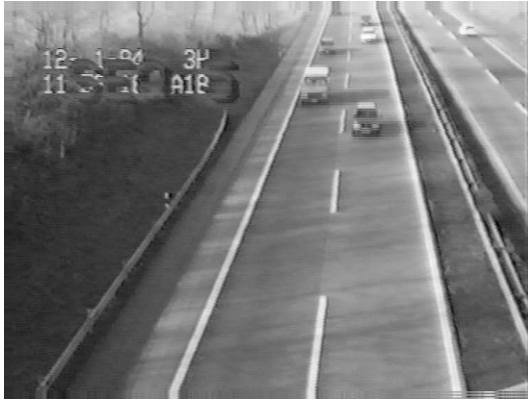
Fig. 1. A traffic surveillance example. This is a typical camera image from a traffic surveillance camera. Notice that especially for dark coloured cars intensity differences between foreground and background are small. In order to track the cars robustly it is necessary to detect the shadows as well as the cars.
