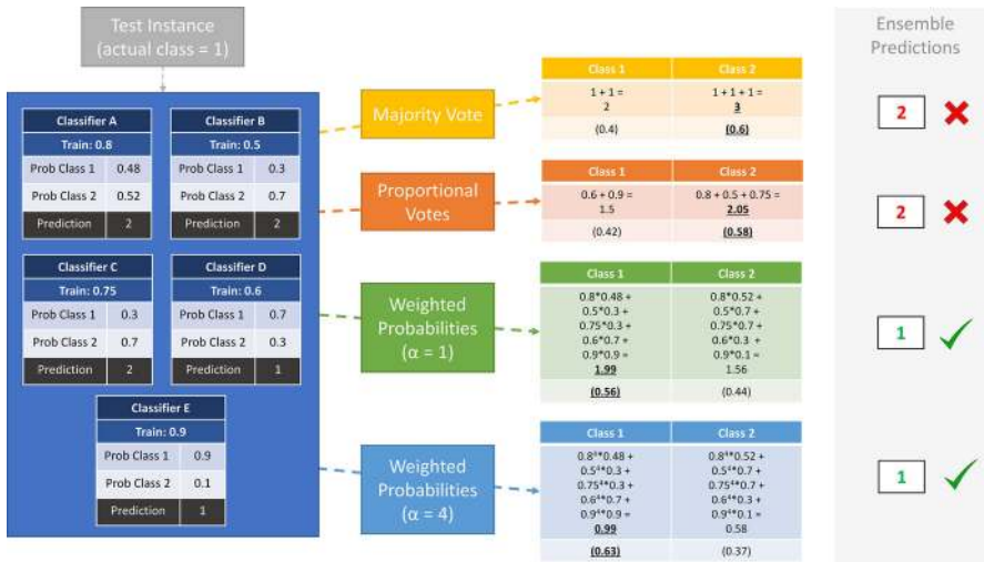
Fig. 1 Illustration of the different effects of combination and weighting schemes on a toy instance classification. Each stage progressively pushes the predicted class probabilities further in the correct direction for this prediction
