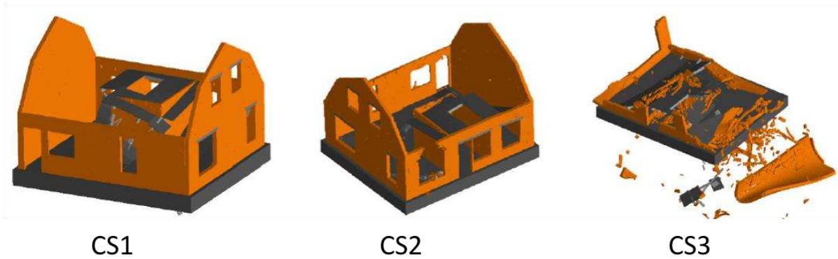
Figure 13. Collapse states observed in an unreinforced masonry numerical model during three different nonlinear dynamic analyses
