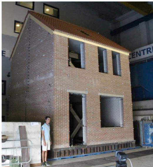
346 Figure 7. Left: Terraced house full-scale specimen on shake-table; Right: observed damage pattern 347 (Graziotti et al. 2017a)
