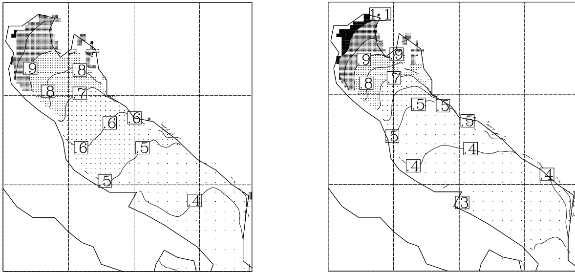
Fig. 7. Maximum surge recorded in the time-slice experiment. Model simulations of the present (left) and doubled- \text{CO}_2 (right) climates are shown
