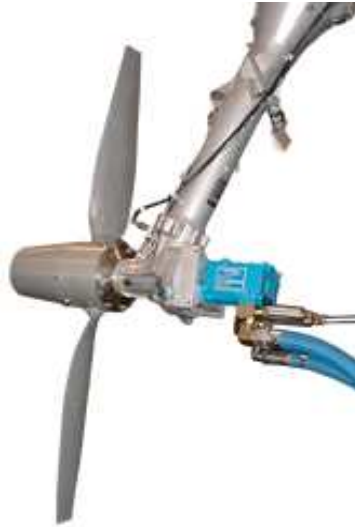
Figure 64: Ram Air Turbine [87]
