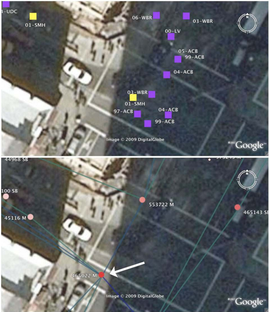
Fig. 8 Top : ECS tickets located near MH 465022. Bottom : Structures and Cables near MH 465022. A white arrow indicates the position of MH 465022
