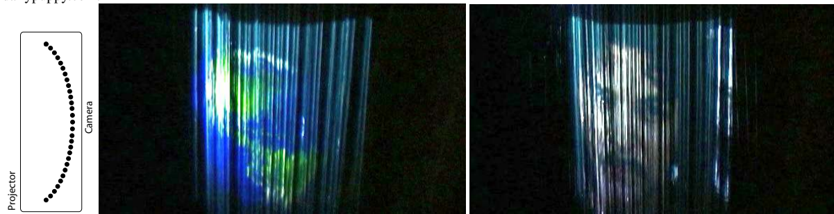
(d) Curved display: Four emitters and a thin-plate spline were used to calibrate this 41 emitter display. Any object that can be approximated by a vertically-constant curve can be projected with such a display, such as a globe or the face of Inigo Montoya from The Princess Bride .
