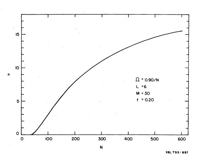
Fig. 4. The number of counters, n, without pile-up and no neighbor counters firing as a function of the total number of counters, N, with a total efficiency of 90%, a multiplicity of 30, f = 0.2, and six nearest neighbors for each crystal.
