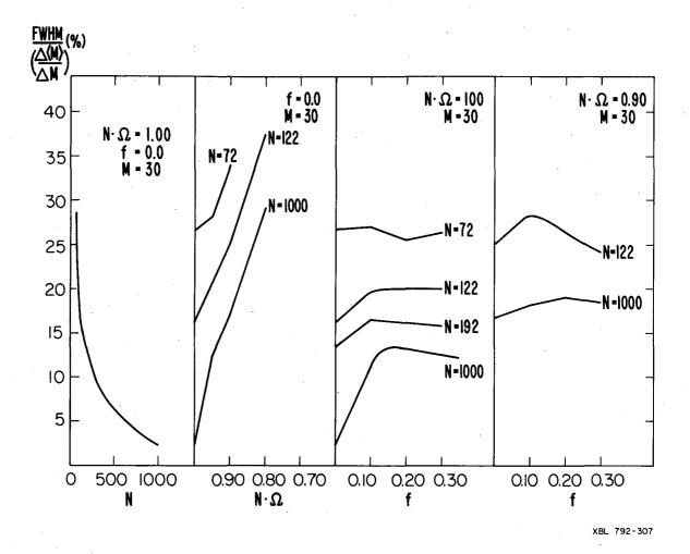
Fig. 2. The multiplicity resolution (the FWHM in percent divided by  $\Delta < M > /\Delta M$ , the ratio between the difference of the measured average multiplicity and the original differences) as a function of the number of counters, N, the total efficiency N· $\Omega$ , and the probability for Compton scattering between one crystal and its neighbors, f.
