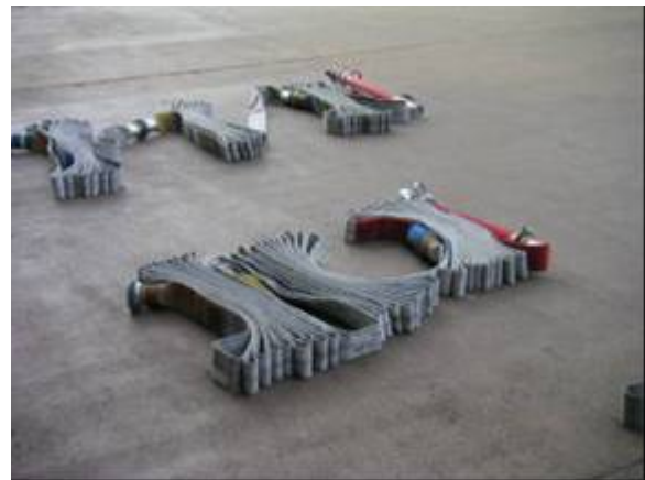
Fig.7 Folded water hose for fire extinguisher
