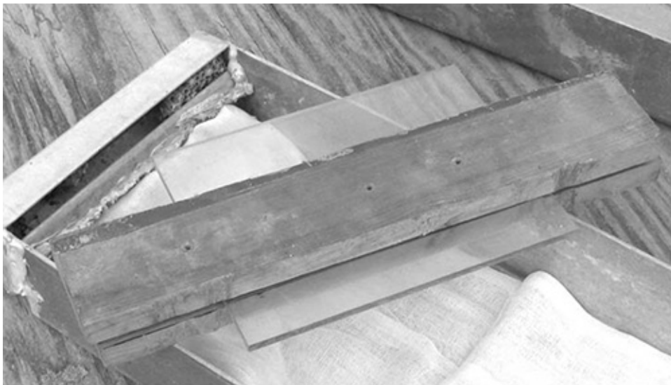
Figure 2. Box packing materials. Approximately 4 layers of cheesecloth in the bottom of the box prevent soil loss but allow water to drain freely. A leveling gauge consisting of acrylic glass sandwiched between two wooden boards is as wide as the box (20 cm) and as deep (2.5 cm) as the difference between the sides of the box (7.5 cm) and the top of the gutter (5 cm). By resting the board on the lip of the box the acrylic glass is used to grade soil to the depth of the gutter.
