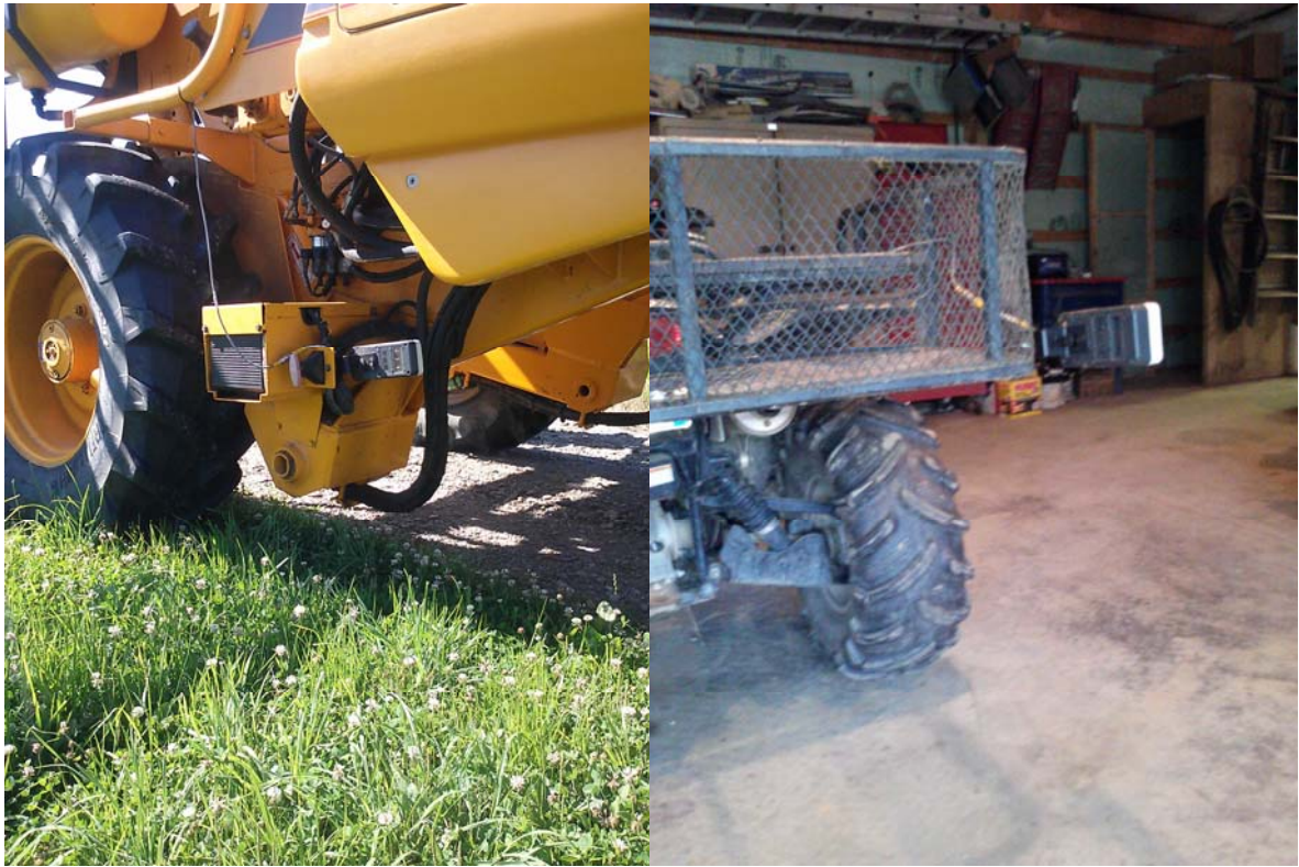
Figure 3 Examples of mounting of the Crop-Circle sensor on a (left) harvester-sprayer and (right) an all-terrain vehicle.
