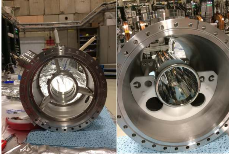
Figure 3: Photographs of: (left) the second set of decelerating electrodes, mounted in their 250CF vacuum chamber on MACOR ® stand-offs; (right) the pulsed drift tube, machined from stainless steel, mounted on a MACOR ® “cradle” for stability and insulation.
