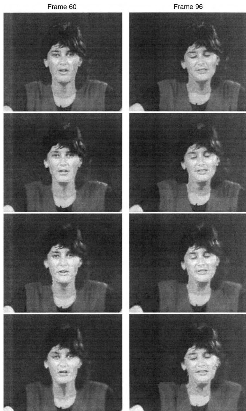
Fig. 11. Coder performance for Miss America sequence at different bit-rates. In the order from top to down, original frames and coded frames at 37, 23 and 16 kbit/s, respectively.
