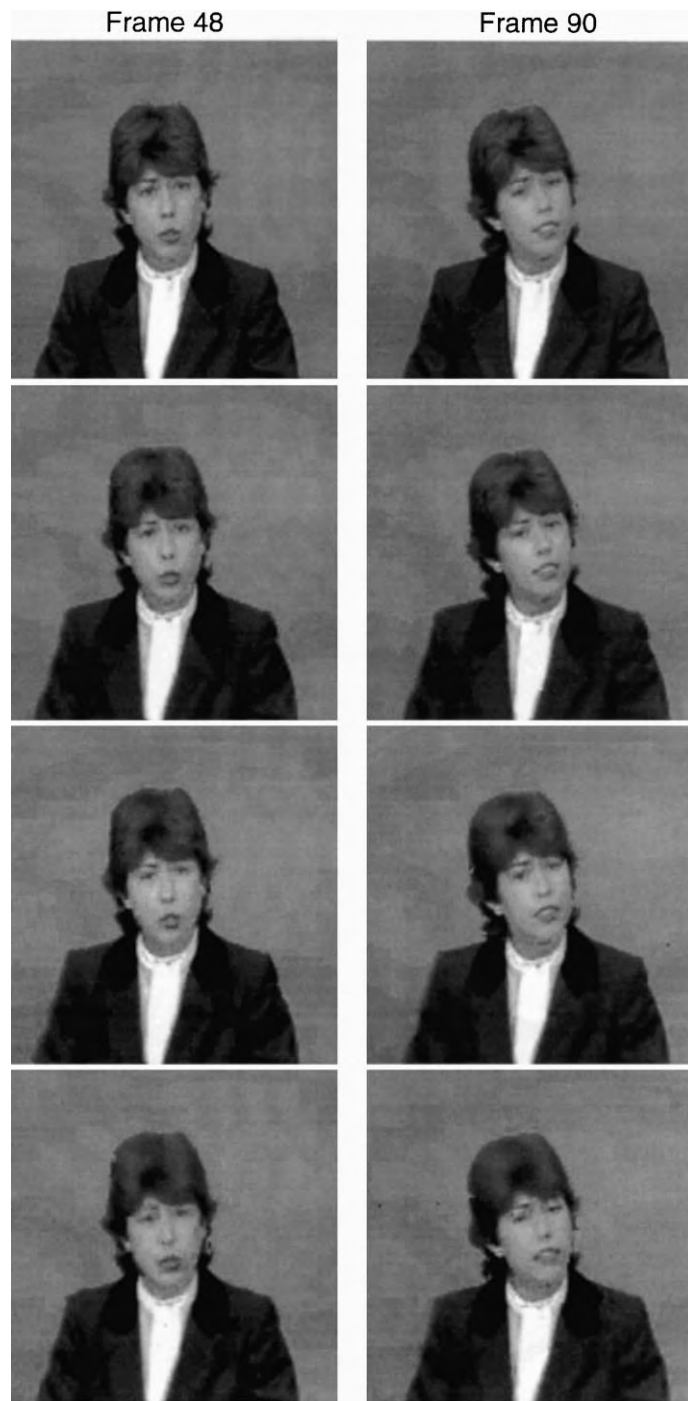
Fig. 12. Coder performance for Claire sequence at different bit-rates. In the order from top to down, original frames and coded frames at 36, 28 and 17 kbit/s, respectively.
