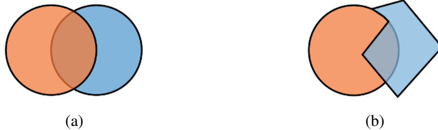
Figure 2.3 Two overlapping objects. (a) A simple overlap occurring at two boundary points and (b) an overlap along a boundary edge and a single boundary point.
