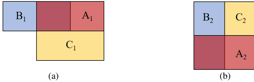
Figure 1.4 Two distinct configurations that map onto the same binary relations using 4-intersection or RCC-8. First, (a) A and B overlap , C meet A and B, and (b) A and B overlap , C meet A and B.
