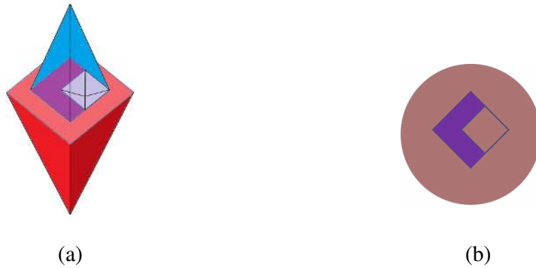
Figure 6.3 Two volumes intersect in two alternate views. (a) A diagram of their intersection and (b) a representation of the bottom object's boundary as a disk, with its intersection with the upper object.
