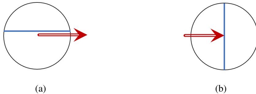
Figure 4.7 Two distinct edge sequences. (a) One line begins within the interior of a second line and (b) one line touches the interior of another line and ends.
