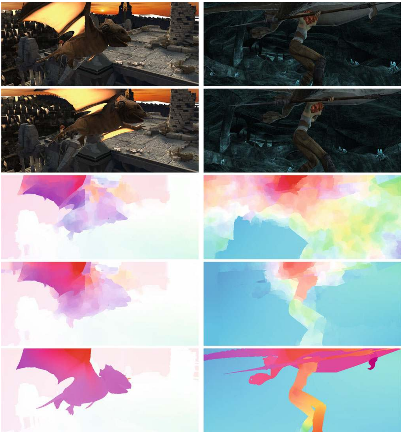
Fig. 10 Example results on MPI Sintel dataset. From top to bottom : first frame, second frame, results by Classic+NL (5-level), results by Classic+NLP (7-level), and ground truth. The asymmetric pyramid leads to a significant improvements in large regions undergoing large motion (head of the dragon on the left and background on the right ).
