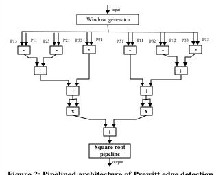
Figure 2: Pipelined architecture of Prewitt edge detection
