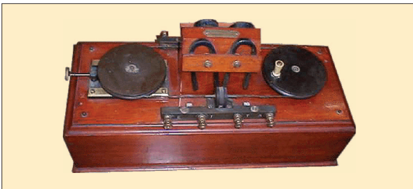
FIGURE 4 – A Marconi magnetic detector, developed in 1902. (Photo courtesy of Spark Museum.)
