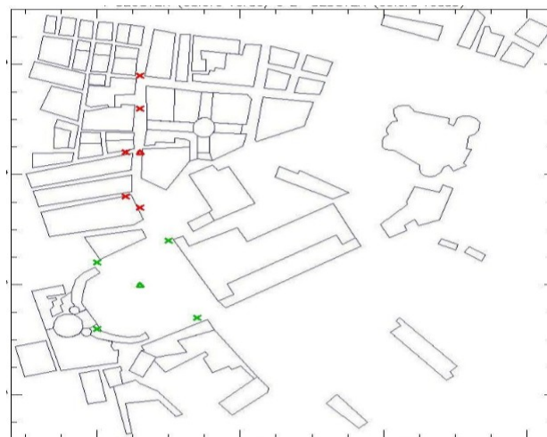
Fig. 5. WSN in the area of Naples city centre. Cluster A (green) and cluster B (red) nodes (crosses) and gateways (triangles).
