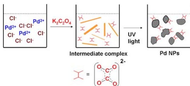
Fig. 7 Schematic representation of the formation of Pd nanoparticles by the photochemical decomposition method
