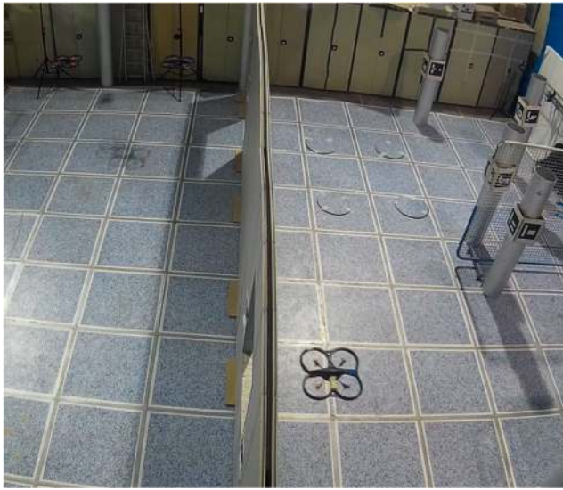
Fig. 21 Real flight experiment of [36], using the previous version of the here presented path planning solution for a multi-robot search and rescue application
