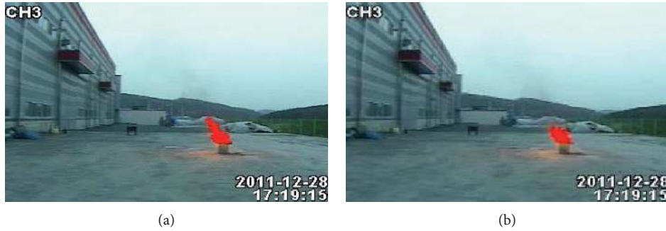
FIGURE 8: The number of fire pixels in adjacent frames. There are 1,784 fire pixels in (a) and 1,465 in (b).
