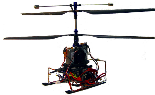
Fig. 1. The helicopter used in this work. It is based on E-flite Blade CX2, a coaxial 4-channel indoor RC helicopter (gross weight: 224 g, rotor span: 345 mm). Modifications include: (1) removal of the original canopy and tail boom to increase payload; (2) adding a metal frame with 5 LEDs as feature points in video tracking.
