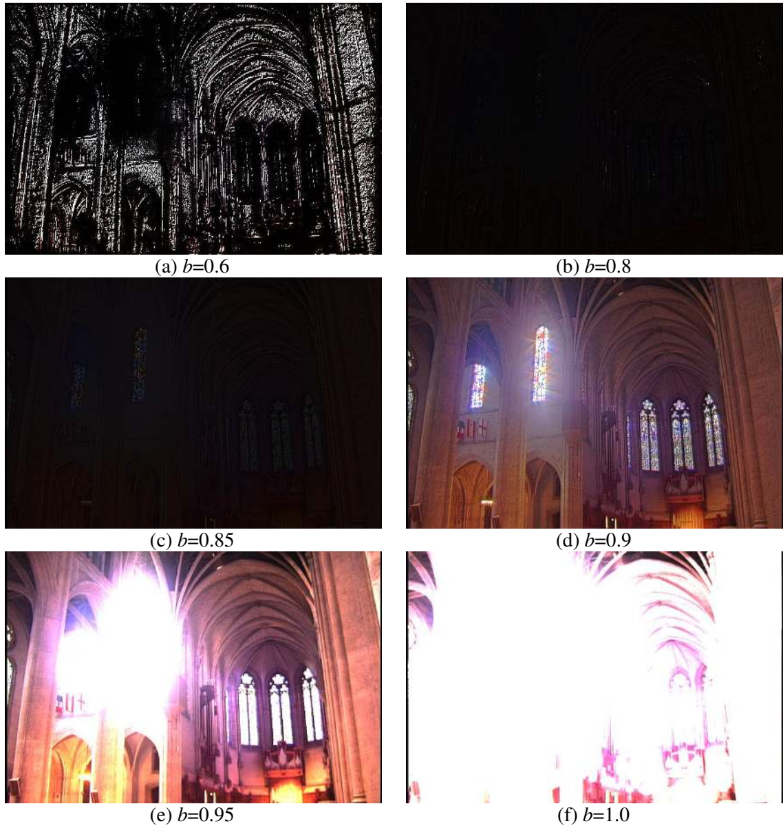
Figure 4.2 Experiment showing the effect of the parameter b on the tone mapping of the dynamic range of the Nave image.
