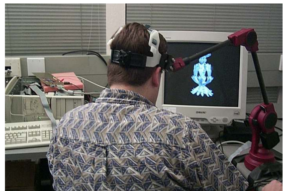
Figure 3. Using the light field renderer. Note the mechanical arm tracking the user's head and the PC in the background which contains the custom hardware for the renderer.
