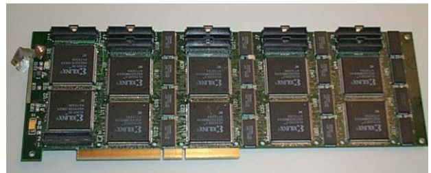
Figure 6 The PARTS board. Additional FPGAs are located on the other side of the board.
