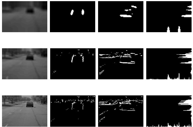
Fig. 3. Multi-scale hypothesis generation. The sizes of the images in the first row are: 90 \times 62 ; the second row: 180 \times 124 ; and the third row: 360 \times 248 . The images in the first column are the ones after low pass filtering in different scales; the second column: vertical edge maps; the third column: horizontal edge maps; and the fourth column: vertical and horizontal profiles. For illustration purposes, all the images have been scaled back to 360 \times 248
