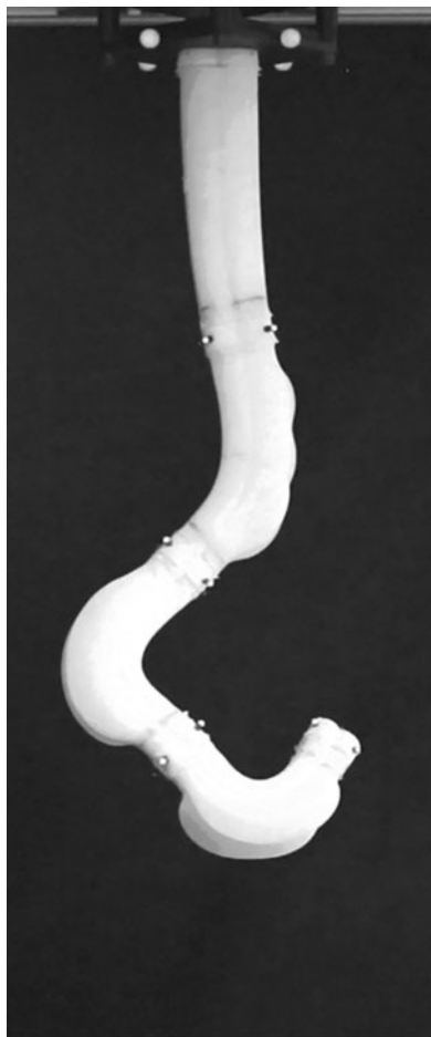
FIG. 21. A spatial cylindrical soft manipulator prototype.
