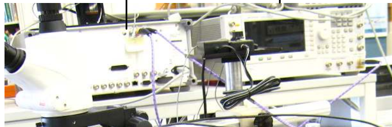
Fig. 3.11. Using a 40GHz signal generator in combination with the upconverter of another signal generator to produce a 60GHz signal
