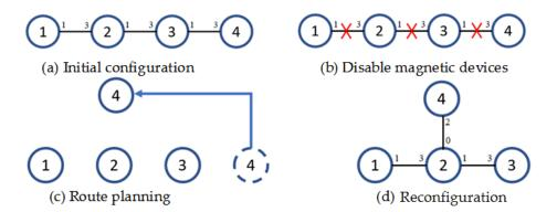
Figure 11. Modular vehicle configuration reorganization process.
