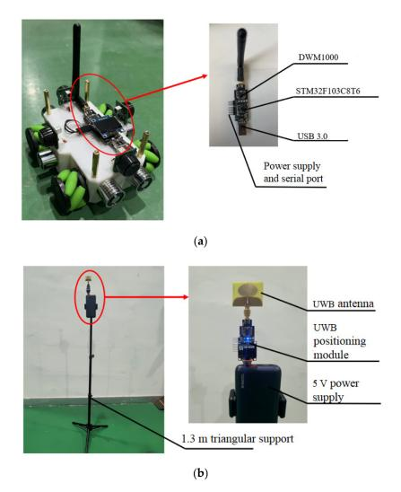
Figure 8. (a) Positioning module on modular car; (b) Positioning module on base station.
