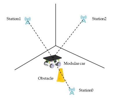
Figure 5. UWB positioning system.
