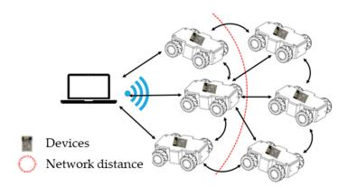
Figure 4. ESP-MESH of modular vehicles.
