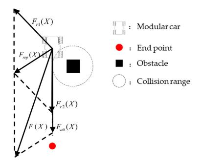
Figure 9. Force analysis of improved artificial potential field method.
