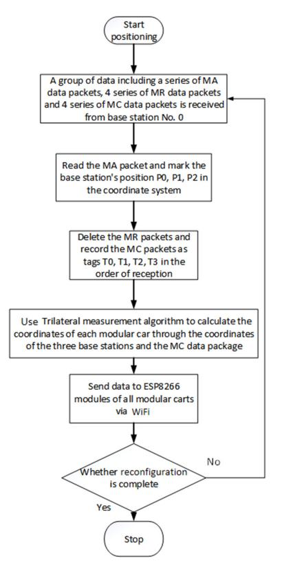
Figure 14. Flow chart of UWB location algorithm.
