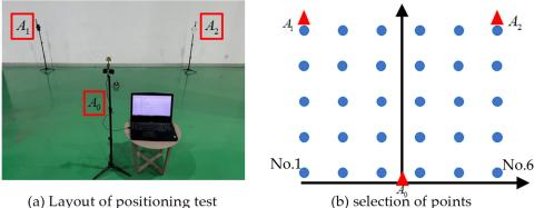
the selection of the positioning points divides the entire plane into 30 positioning points. The interval between each positioning points is 0.6 m, as shown by blue dots in Figure 15b.
