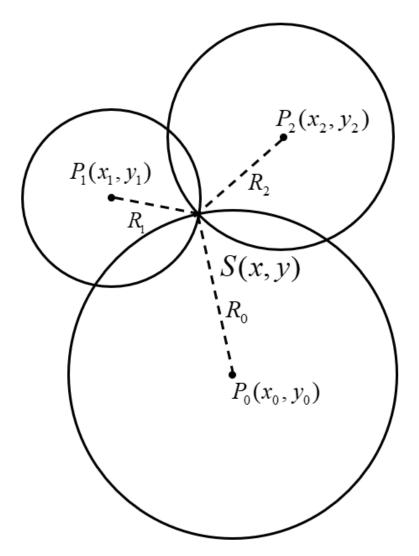
Figure 7. Trilateral measurement algorithm.
