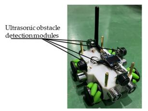
Figure 3. Ultrasonic obstacle detection modules.
