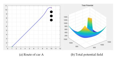
Figure 18. Single modular vehicle path under improved artificial potential field method.
