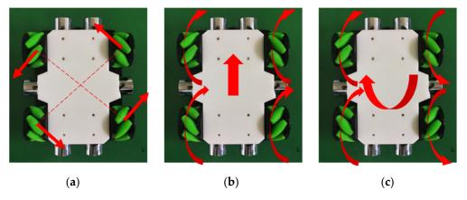
**Figure 1.** Mecanum wheel and layout of wheels: (a) Direction of rollers; (b) Forward movement; (c) Rotational movement.
