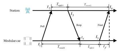
Figure 6. Bidirectional bilateral ranging
