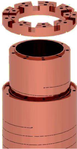
FIGURE 3. A Polyhelix insert. The helices are actually copper alloy tubes cut by a spark erosion technique. Epoxy glue may be introduced into the slit to ensure the electrical insulation between turns : this is the so-called “Longitudinally cooled helices” as the water flow is “longitudinal”. An another possibility to ensure electrical insulation is to introduce periodically some insulators into the slit : this is the so-called “Radially cooled helices” as the water may flow from the inner to the outer radius through the open slit.
