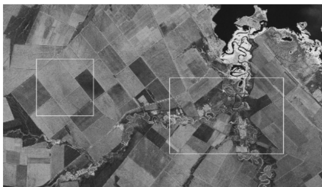
FIGURE 10. TerraSAR-X image used for experiments, of which is acquired by the SM mode of X-band TerraSAR-X over the Volga region of south Russia on June 19, 2007. The resolution is 3 meter, and the polarization is HH, the effective number of looks is 8.3.
