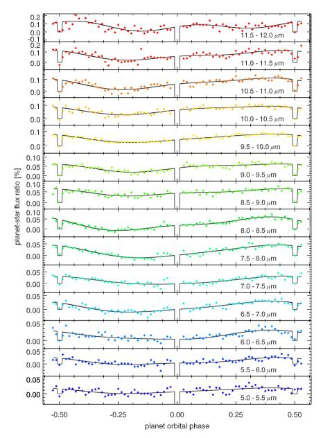
Extended Data Fig. 1 MIRI spectroscopic light curves from 5 to  $12\,\mu\mathrm{m}$ . Black lines are the best-fit astrophysical model to the data, assuming a second-order sinusoid functional form for the phase variation. Colored points are the data binned every 5 degrees in orbital phase, plotted without error bars for clarity. Wavelength ranges for each light curve are as indicated. Note the differing y-axis scale on each sub-panel.
