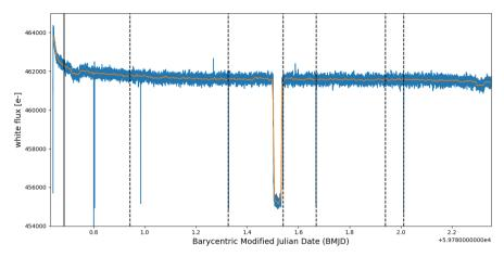
Extended Data Fig. 3 Raw white light curve for GJ 1214b. All the individual integrations are shown in blue. A median filtered (64 points) version of the light curve is shown in orange. For our analysis we discard the 550 integrations (63 min) before the vertical black line. Note the higher discrepant integrations, some of which correspond to HGA moves (vertical dashed lines); the ramp at the start of observations; and the pre-transit brightening.
