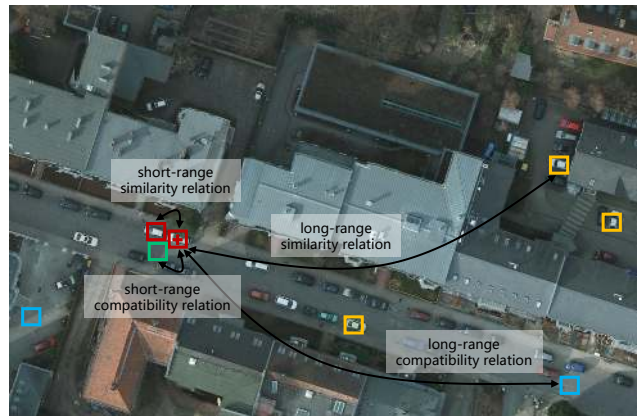
Figure 1: Illustration of long-range spatial relations in an aerial image. Appearance similarity or semantic compatibility between patches within a local region (red–red and red–green) and patches in remote regions (red–yellow and red–blue) underlines our global relation modeling.
